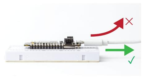
The u.FL antenna connector is a very fragile piece of hardware (and is fancy too with all the gold plating). The connector was not designed to be constantly plugged and unplugged. Care must be
