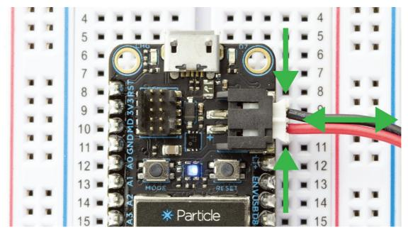
The micro B USB connector on the Argon is soldered on the PCB with large surface pads as well as couple of through hole anchor points. Despite this reinforcement, it is very easy to rip out the connector if too much stress is put on in the vertical direction.
