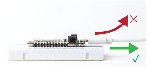
The u.FL antenna connector is a very fragile piece of hardware ( and is fancy too with all the gold plating). The connector was not designed to be constantly plugged and unplugged. Care must be
