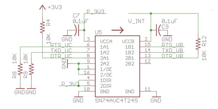
Since u-blox module's communication interface operates at 1.8VDC, while the STM32F205RGT6 microcontroller operates at 3.3VDC, we need voltage translators in-between them. This is achieved with two SN74AVC4T245 non-inverting buffers. The default state of the USART pins is set with the help of pull-up and pull-down resistors, and the unused input pins are tied to GND.
