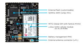
Particle E Series modules 36.0 x 43.0 x 4.6 mm
