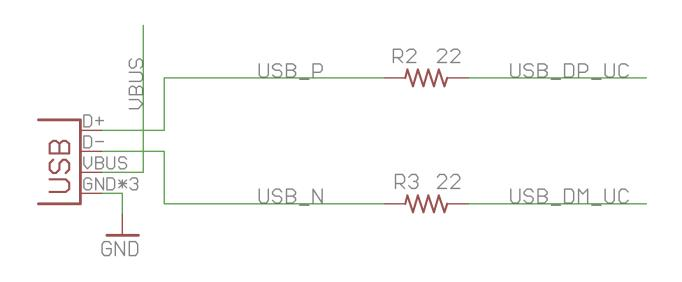
The USB data lines are terminated with 22 Ohm resistors. These data pins are also exposed via small through holes next to the USB connector and are labeled D+ and D-. The VBUS (+5VDC VCC of the USB port) is fed to the PMIC via a 3Amp Schottky diode (SS3P3). The VBUS pin is also available via the unpopulated header hole on the top-right side of the E series.
