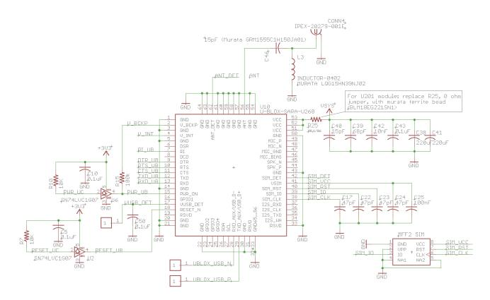
The u-blox cellular module talks to the microcontroller over a full-duplex USART interface using a standard set of AT commands. The eSIM chip is directly connected to the u-blox. The power to the eSIM chip is also provided by the cellular module.
