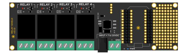
We have even provided a small prototyping area around the shield for you to add more components or connectors. A temperature sensor to go along with your brewer, maybe?
