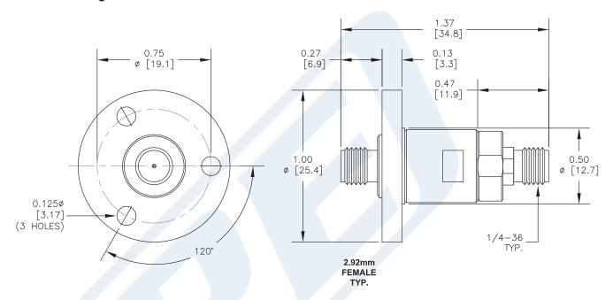
Rotary Joint Operating to 18 GHz 2.92mm Female 2.92mm Female Connectors from Pasternack Enterprises has same day shipment for domestic and International orders. Our RF, microwave and millimeter wave products maintain a 99% availability and are part of the broadest selection in the industry.
