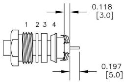
Click the following link (or enter part number in "SEARCH" on website) to obtain additional part information including price, inventory and certifications: N Male Connector Clamp/Solder Attachment for RG213, RG214, RG8, RG9, RG11, RG225, RG393, RG144, RG216, RG215 PE4062
