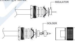
Click the following link (or enter part number in "SEARCH" on website) to obtain additional part information including price, inventory and certifications: N Male Connector Clamp/Solder (Captive Contact) Attachment for RG213, RG214, RG8, RG9, RG11, RG225, RG393, RG144, RG216, RG215 PE4132
