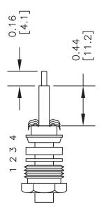
INSERT PTFE BEFORE CONTACT. NOTE: RG62 USES PTFE INSERT TAPER END FIRST.
