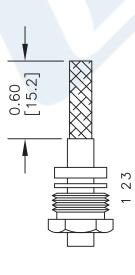
CENTER CONDUCTOR, SOLDER CONTACT TO CENTER 2. FORM BRAID OVER CLAMP NUT (4). TRIM BRAID BACK CONDUCTOR TO DIMENSION SHOWN. DO NOT NICK OVER HEAT DIELECTRIC. INSERT CABLE ASSEMBLY CONDUCTOR. REMOVE EXCESS SOLDER. DO NOT TO SHOULDER. CUT DIELECTRIC & CENTER INTO BODY & TIGHTEN.
