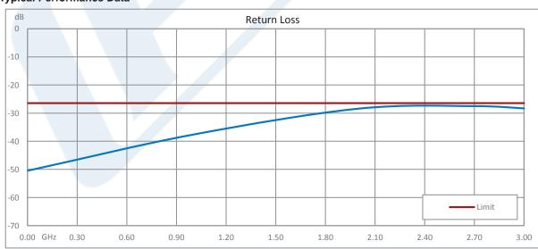
Click the following link (or enter part number in "SEARCH" on website) to obtain additional part information including price, inventory and certifications: 50 Watt RF Load Up to 3 GHz With N Female Input Round Body Black Anodized Aluminum Heatsink PE6234
