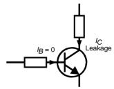
Leakage current Ic=0.17mA
