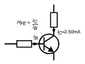
The gain of all transistors can vary considerably with collector current, collector voltage and also temperature. The displayed value for gain therefore may not represent the gain experienced
