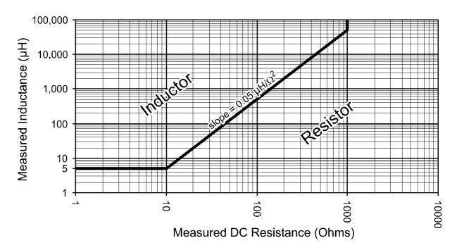
For example, if the inductance of your component is measured at  $100\mu H$  and it has a DC resistance of  $100\Omega$ , then the Atlas LCR will tell you that you have a resistor. If however the resistance was only  $10\Omega$ , then the Atlas LCR will you that you have an inductor.
