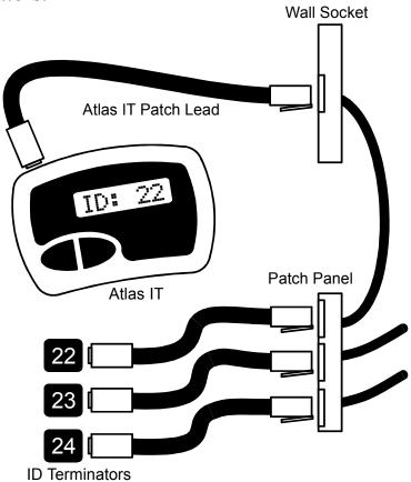
These special terminators can be used in exactly the same way as the standard (non-identified) terminators. They are automatically recognised by the *Atlas IT*
