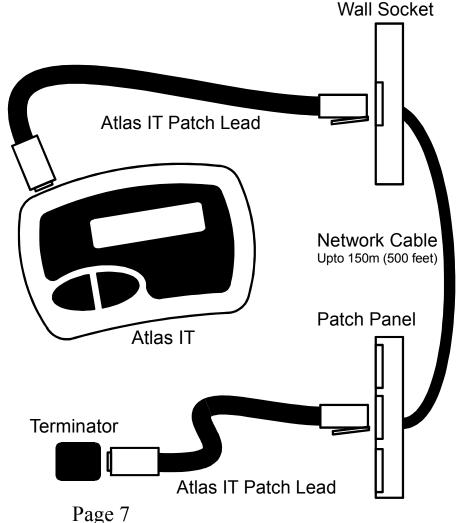
The *Atlas IT* can only provide useful information if the cabling being tested is not connected to other active equipment (such as computers, hubs and routers). Only the *Atlas IT* and the *Atlas IT* Terminator should be connected to the cabling.
