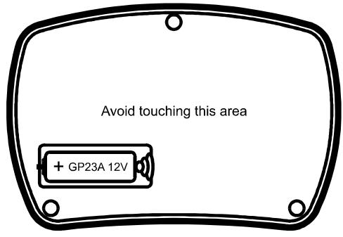
The battery should be replaced with a high quality battery identical to, or equivalent to an Alkaline 23A, V23A, GP23A, MN21 12V (10mm diameter x 28mm length). Carefully replace the rear panel, do not over-tighten the screws.
