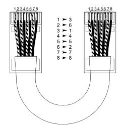
Please note, there are actually a number of wiring configurations that can be used to produce a crossover cable. The cable connection pattern shown above is the most common.
