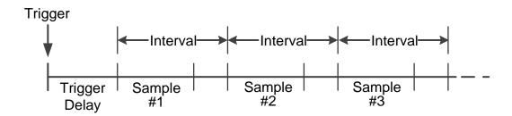
Set the trigger delay time: Press the Delay softkey to select Manual, press to move the cursor, press to increase or decrease the value. The range is 1 ms to 999.999 ms.
