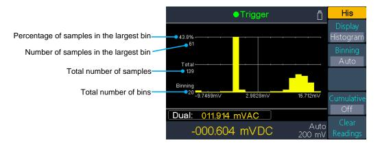
Press the Binning softkey to select Auto binning or Manual binning.
