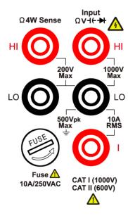
The user-replaceable 10 A current-protection fuse is on the front panel. To maintain protection, replace fuse only with fuse of the specified type and rating. About the specified type and rating of the fuse, please refer to "7 Current Terminal Fuse" in "Front Panel Overview" on page 9.
