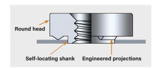
A variety of welding equipment is suitable for installation of PEM® weld nuts. Best results have been obtained with a 50KVA press-type, spot-welding machine whose upper welding head moves vertically in a straight line with the lower electrode. Flat-faced electrodes with tip diameters .125" / 3.2 mm larger than the "E" dimension of the PEM® weld nut should be used.
