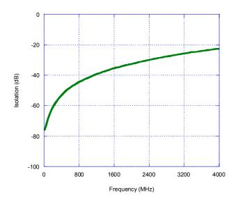
Figure 9. Isolation - RF1 to RF2, RF2 to RF1
