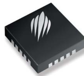
Figure 2. Package Type 20-lead 4x4mm QFN
