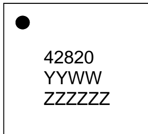
Figure 17. Top Marking Specification
