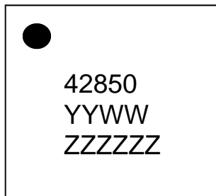
Figure 26. Top Marking Specification
