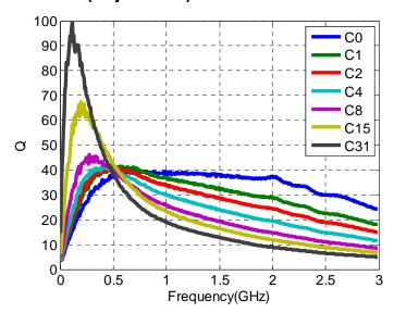
Figure 9. Measured Shunt Q vs State
