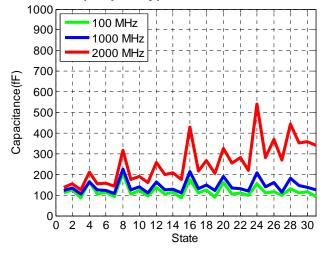
**Measured Shunt C vs Frequency** Figure 7. (major states)
