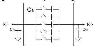
Shunt configuration (looking into RF+ when RF- is grounded) will have higher total capacitance at RF+ due to parallel combination of C<sub>S</sub> with parasitic capacitance C<sub>P1</sub> (C<sub>S</sub> + C<sub>P1</sub>), as demonstrated in Figure 15 and Table 9.
