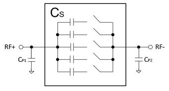
Shunt Configuration (looking into RF+ when RF- is grounded) will have higher total capacitance at RF+ due to parallel combination of Cs with parasitic capacitance  $C_{P1}$  ( $C_S + C_{P1}$ ), as demonstrated in *Figure 14* and *Table 9.*
