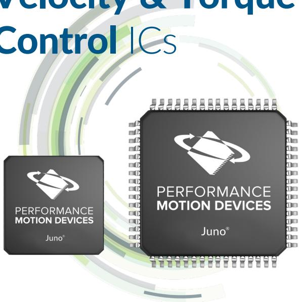
**The Juno Family of ICs** provide advanced velocity and torque control for Brushless DC, DC Brush, and step motors. They are the industry's first family of compact ICs with full four quadrant motion control, direct input quadrature encoder, profile generation, and advanced current control.
