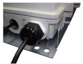
5) Thread outdoor rated waterproof AC cable (must comply with all local, national and country electrical codes) from source through piping/gland to the terminal block. The AC cable will need to be a minimum of 14AWG and terminated with M3.5 spade lugs. Pair
