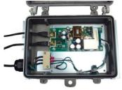
7) Reattach the protective covering over the PC board and terminal blocks and re-close the lid. Ensure that the four captive screws are fully tightened before operation can commence.
