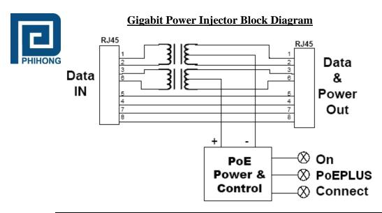
**Description of LED Functions for Gigabit Power Injector**
