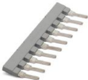
Insertion bridge, pitch: 15.25 mm, number of positions: 10, color: gray
