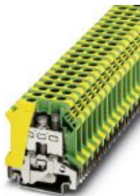
Ground terminal block with screw connection, cross section: 0.5 ... 6 mm 2 , AWG: 20 ... 8, width: 8.2 mm, color: green...yellow
