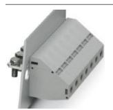
Panel feed-through terminal block, connection method: Screw connection with tension sleeve, Cable lug connection, number of positions: 1, load current: 150 A, cross section: 16 mm² - 50 mm², connection direction of the conductor to plug-in direction: -90 °, width: 18.8 mm, color: gray
