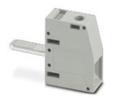
Panel feed-through terminal block, connection method: Screw connection with tension sleeve, Screw connection with tension sleeve, number of positions: 1, load current: 150 A, cross section: 16 mm² - 50 mm², connection direction of the conductor to plug-in direction: 0 °, color: gray
