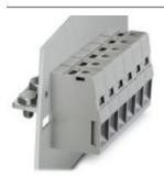
Panel feed-through terminal block, connection method: Screw connection with tension sleeve, Cable lug connection, number of positions: 1, load current: 232 A, cross section: 35 mm² - 95 mm², connection direction of the conductor to plug-in direction: 0 °, width: 25 mm, color: gray
