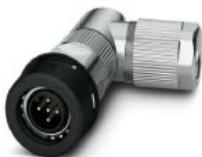
Connector, Universal, 5-position, shielded, Plug angled M12 Push-Pull, Coding: A, Crimp connection, knurl material: PA 6.6, external cable diameter 4.5 mm ... 7.5 mm, without crimp contacts
