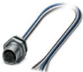
Sensor/actuator panel-mount connector, 5-pos., M12 push-pull, A-coded, rear/screw mounting with M16 thread, with straight solder connection
