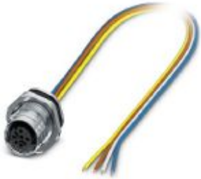
Sensor/actuator panel-mount connector, 4-pos., M12 push-pull, D-coded, rear/screw mounting with M16 thread, with straight solder connection
