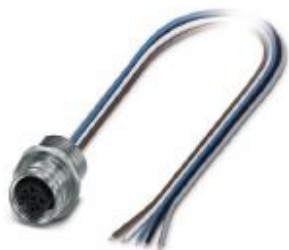
Sensor/actuator panel-mount connector, 5-pos., M12 push-pull, A-coded, front-wall/screw mounting with M16 thread, with straight solder connection
