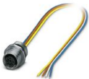
Sensor/actuator panel-mount connector, 4-pos., M12 push-pull, D-coded, front-wall/screw mounting with M16 thread, with straight solder connection
