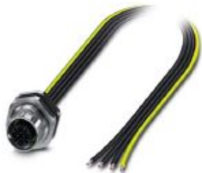
Flush-type connector, Power, 4-position, Socket, M12, S power, Rear mounting, M16 x 1.5, Individual wires, UL/cUL stranded hook-up wire
