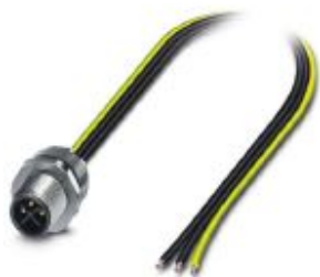
Flush-type connector, Power, 3-position, Plug, M12, S power, Front mounting, M16 x 1.5, Individual wires, PP litz wire
