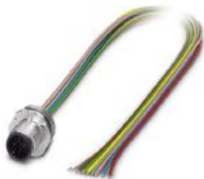
Sensor/Actuator flush-type plug, 8-pos., M12-SPEEDCON, A-coded, front/screw mounting with M16 thread, with 0.5 m TPE litz wire, 8 x 0.25 mm 2
