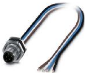
Flush-type connector, Universal, 5-position, Plug, M12, A-coded, Rear mounting, M16 x 1.5, Individual wires, TPE litz wire
