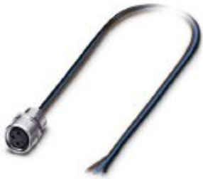
Flush-type connector, 3-position, Socket, straight, M8, Front mounting, M8 x 0.5, Individual wires, cable length: 2 m, 0.25 mm 2 , PVC litz wire
