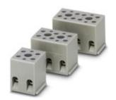
Device terminal block, nom. voltage: 500 V, nominal current: 32 A, connection method: Screw connection, number of connections: 4, number of positions: 2, cross section: 0.2 mm² - 4 mm², AWG: 24 - 12, width: 20 mm, height: 24 mm, color: gray, mounting type: direct screw connection
