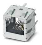
RJ45 PCB connectors, type: RJ45, degree of protection: IP20, number of positions: 8, 10 Gbps, connection method: Solder connection
