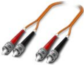
Multi-mode OM1 duplex jumper, ST-ST, UPC polishing, length 10 m
