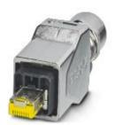
Push-pull ADVANCE connector (version 14), die-cast zinc, with RJ45 connector insert, 8-pos., 10 Gbps,  $CAT6_A$  (IEC 11801:2017), with IDC fast connection technology, for AWG 23 - 22 1-wire, 7-wire, and 19-wire conductors, for cable diameter of 5.5 mm ... 10 mm
