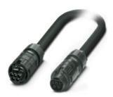
Circular connectors (cable-side), Range of articles: PRC, Connecting cable, housing material: PPE, color: black, number of positions: 5, nom. voltage: 690 V AC, rated current: 32 A, Connection method: Screw connection, Type of contact: Socket/pin
