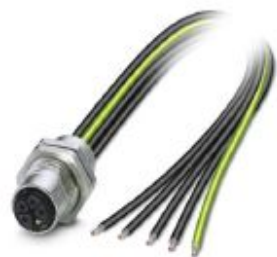
Flush-type connector, Power, 5-position, Socket, M12, K - Power, Rear mounting, M16 x 1.5, Individual wires, cable length: 0.5 m, 2.50 mm 2 , PEX litz wire
