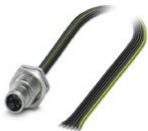
Flush-type connector, Power, 6-position, Plug, M12, M - Power, Rear mounting, M16 x 1.5, Individual wires, cable length: 1.5 m, 1.31 mm 2 , UL/cUL stranded hook-up wire
