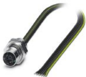
Flush-type connector, Power, 6-position, Socket, M12, M - Power, Rear mounting, M16 x 1.5, Individual wires, cable length: 1.5 m, 1.31 mm 2 , UL/cUL stranded hook-up wire
