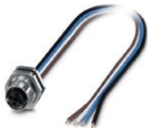
Flush-type connector, Power, 4-position, Socket, M12, T power, Rear mounting, M16 x 1.5, Individual wires, cable length: 0.5 m, 1.31 mm 2 , UL/cUL stranded hook-up wire
