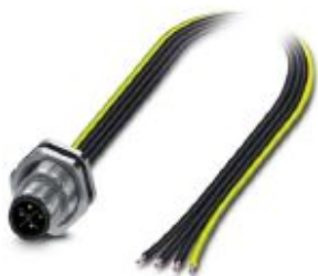
Flush-type connector, Power, 4-position, Plug, M12, S power, Rear mounting, M16 x 1.5, Individual wires, cable length: 1.5 m, 1.31 mm 2 , UL/cUL stranded hook-up wire
